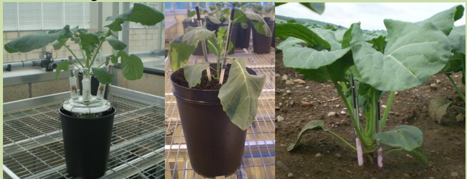
Root volatiles collection from glasshouse- and field-grown broccoli plants using Tenax TA tubes analysed by ATD-GC-MS and in situ SPME analysed by GC-MS.
