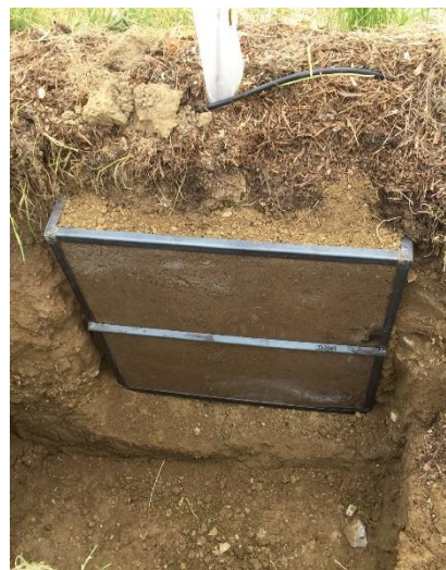
Photograph 4: In situ rhizotron in the apple-agroforestry experiment on plot A1 of the “domaine de Restinclière” (picture by Benjamin Pitchers).
