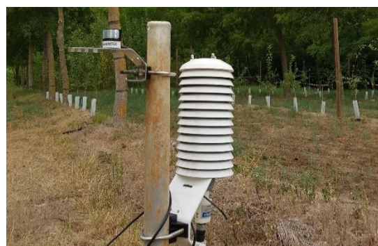
Photograph 1: SP1110 pyranometer (left) and HMP155 in weatherproof housing (right).
